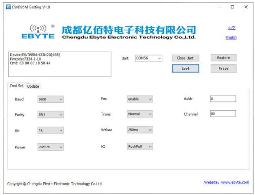
• In the configuration host computer, the radio address, frequency channel, network ID, and key are all displayed in decimal mode, and the value range of each parameter is:
